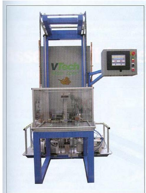
*The VTech (Alpharetta, Georgia, U.S.) MasSpec is an automatic helium leak detector for testing refrigeration components and complete refrigeration units, even in the presence of polyurethane foam. It detects helium leaks as small as 0.1 oz of R-134a per year. It requires just 10% helium concentration at atmospheric pressure. VTech is part of Galileo Vacuum Systems*
