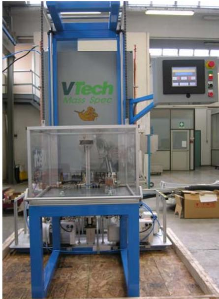
We conducted the first trials with our VTech MasSpec. This is an automatic helium leak detector, based on outside-in technology. The unit under test is evacuated and exposed to a helium mass spectrometer in a containment chamber filled with a small percentage of helium (between 10 and 20%). In case of leaks or microporosities, helium is pulled into the unit and is detected by the mass spectrometer.
