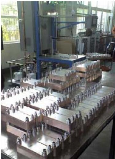
Kaori is currently using the VTech MasSpec for the integral leak detection of their brazed plate heat exchangers. The quality of the leak testing is certified by a calibrated leak and the testing results, thanks to the Data-Logging software accessory, are recorded to a database for data mining and/or print out of testing certificates.
